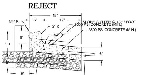
TIE-BAR IF ADJACENT TO CONCRETE (NO.4 X 2'-0" TIE BARS SPACED AT 3'-0" C-C)
