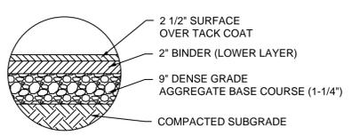
**B ASPHALT PAVEMENT SECTION**
