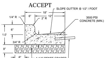
TIE-BAR IF ADJACENT TO CONCRETE (NO.4 X 2'-0" TIE BARS SPACED AT 3'-0" C-C)
