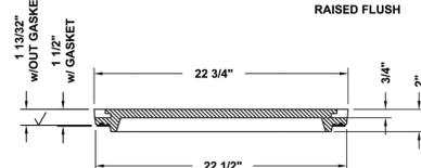
MATERIAL: CAST GRAY IRON ASTM A-48, CLASS 35B
