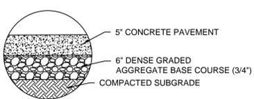
**C CONCRETE SIDEWALK SECTION**
