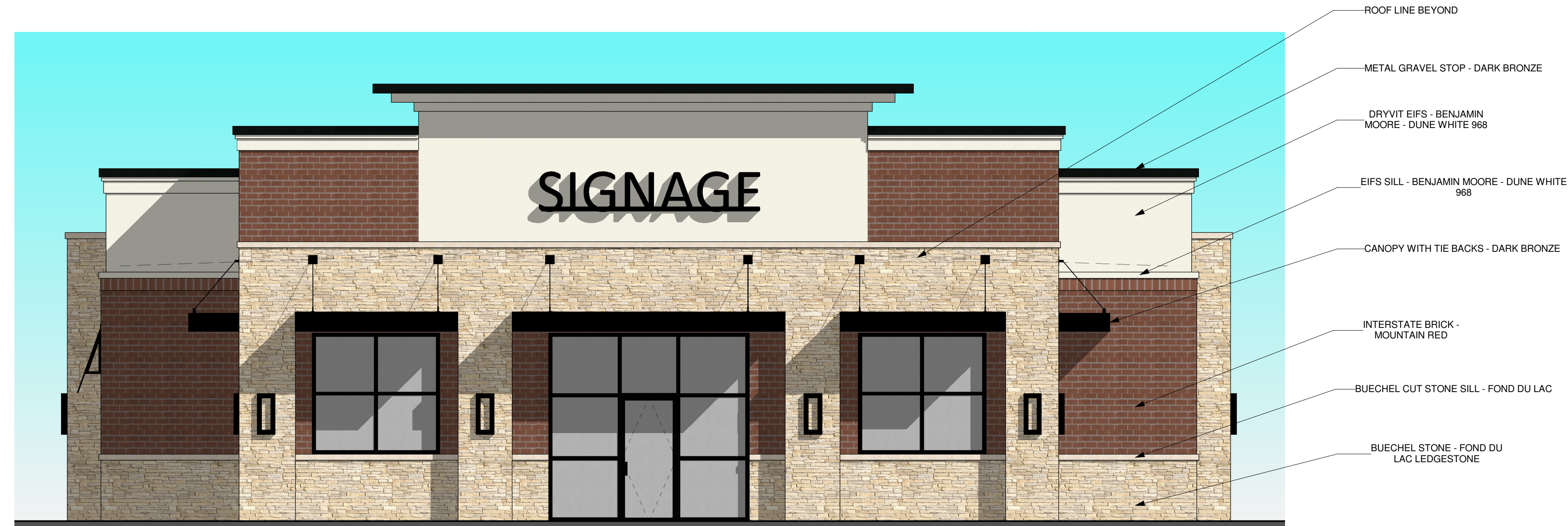
① HEARTLAND DENTAL EAST ELEVATION 1/4" = 1'-0"
