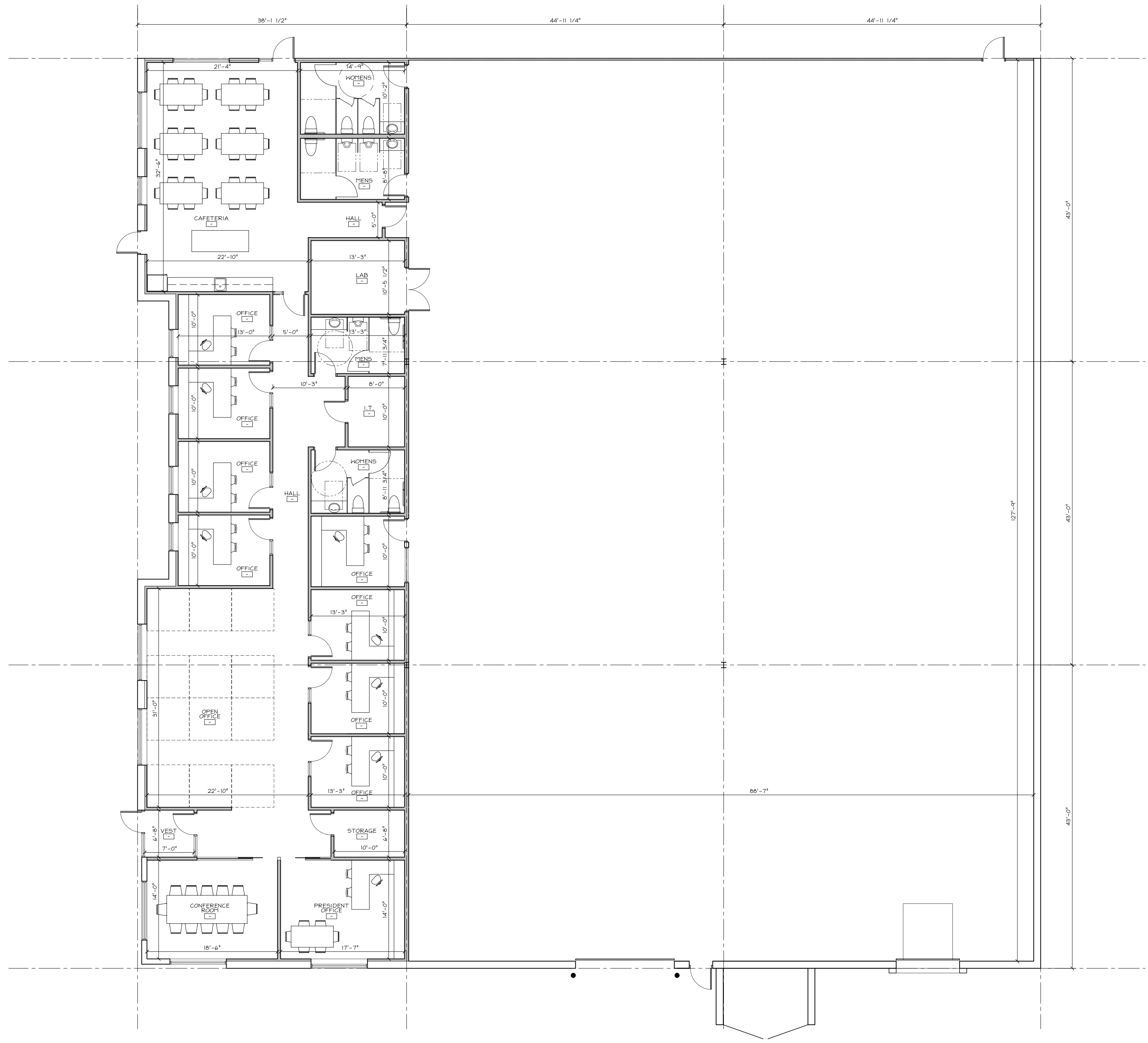
1 FIRST FLOOR PLAN SCALE: 1'-0" = 1/8" OFFICE AREA: 4,119 S.F. WAREHOUSE AREA: 11,956 S.F. TOTAL BUILDING AREA: 16,475 S.F.
