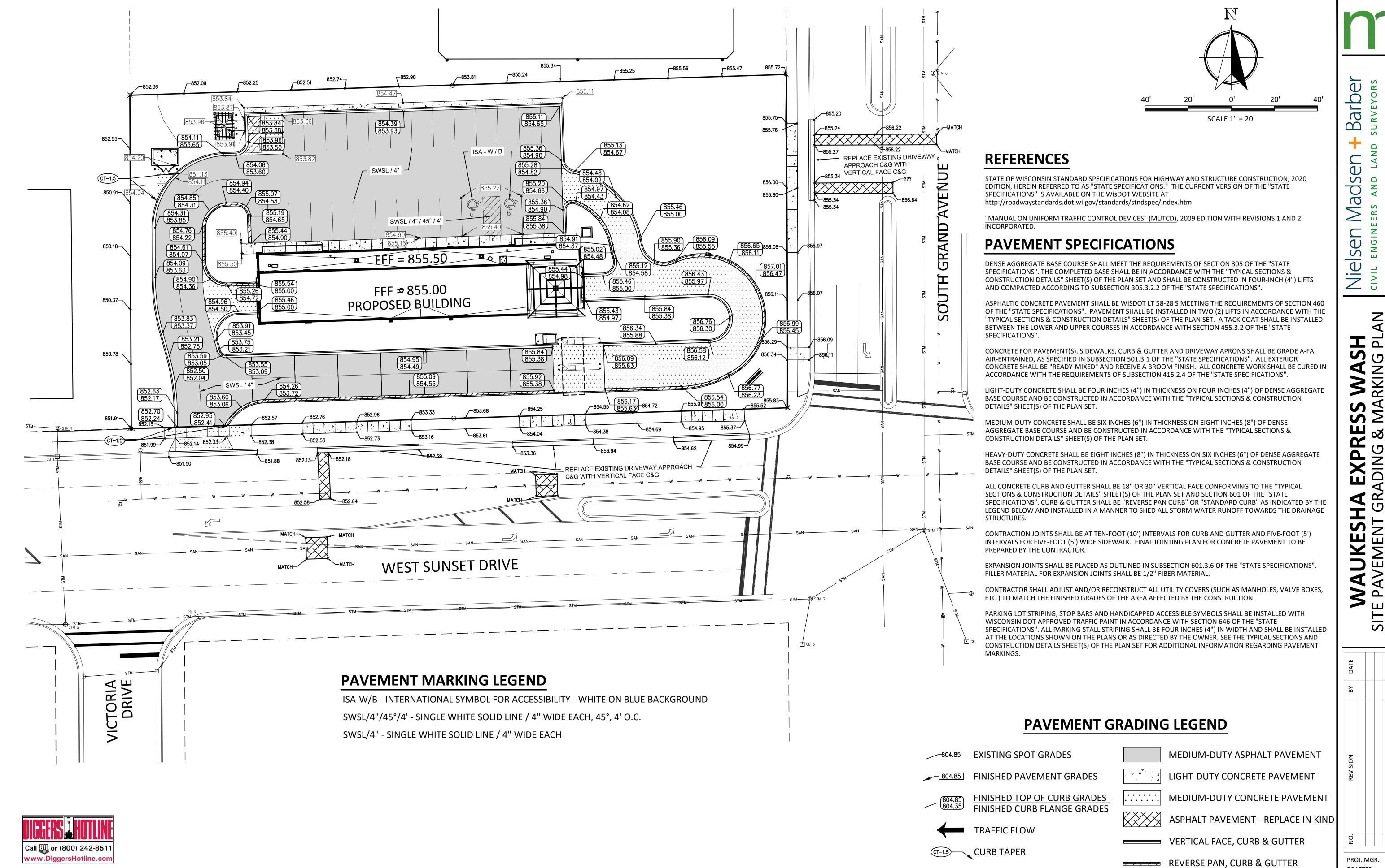
**UTILITY NOTE** EXISTING UTILITIES ARE SHOWN FOR INFORMATIONAL PURPOSES ONLY AND ARE NOT GUARANTEED TO BE ACCURATE OR ALL INCLUSIVE. CONTRACTOR IS RESPONSIBLE FOR VERIFYING THE TYPE, LOCATION, SIZE AND ELEVATION OF UNDERGROUND UTILITIES AS THEY DEEM NECESSARY FOR PROPOSED UTILITY
