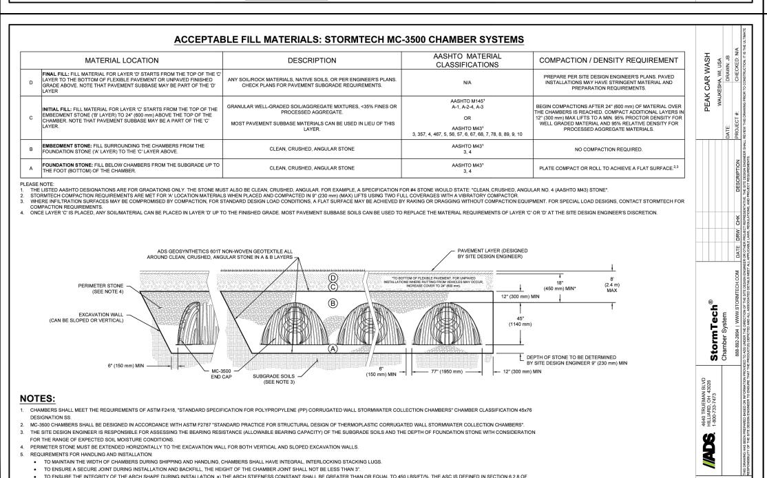
ASTM F2418. AND b) TO RESIST CHAMBER DEFORMATION DURING INSTALLATION AT ELEVATED TEMPERATURES (ABOVE 73° F / 23° C), CHAMBERS SHALL BE PRODUCED FROM REFLECTIVE GOLD OR YELLOW
