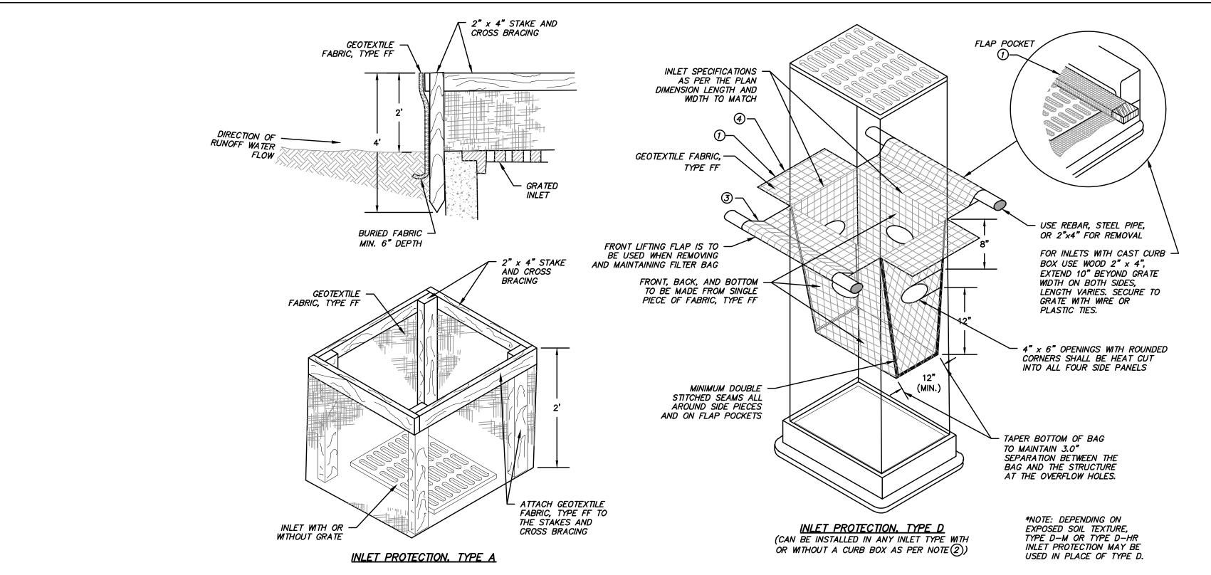
FINISHED SIZE, INCLUDING FLAP POCKETS WHERE REQUIRED, SHALL EXTEND A MINIMUM OF 10" AROUND THE PERIMETER TO FACILITATE MAINTENANCE OR REMOVAL.
