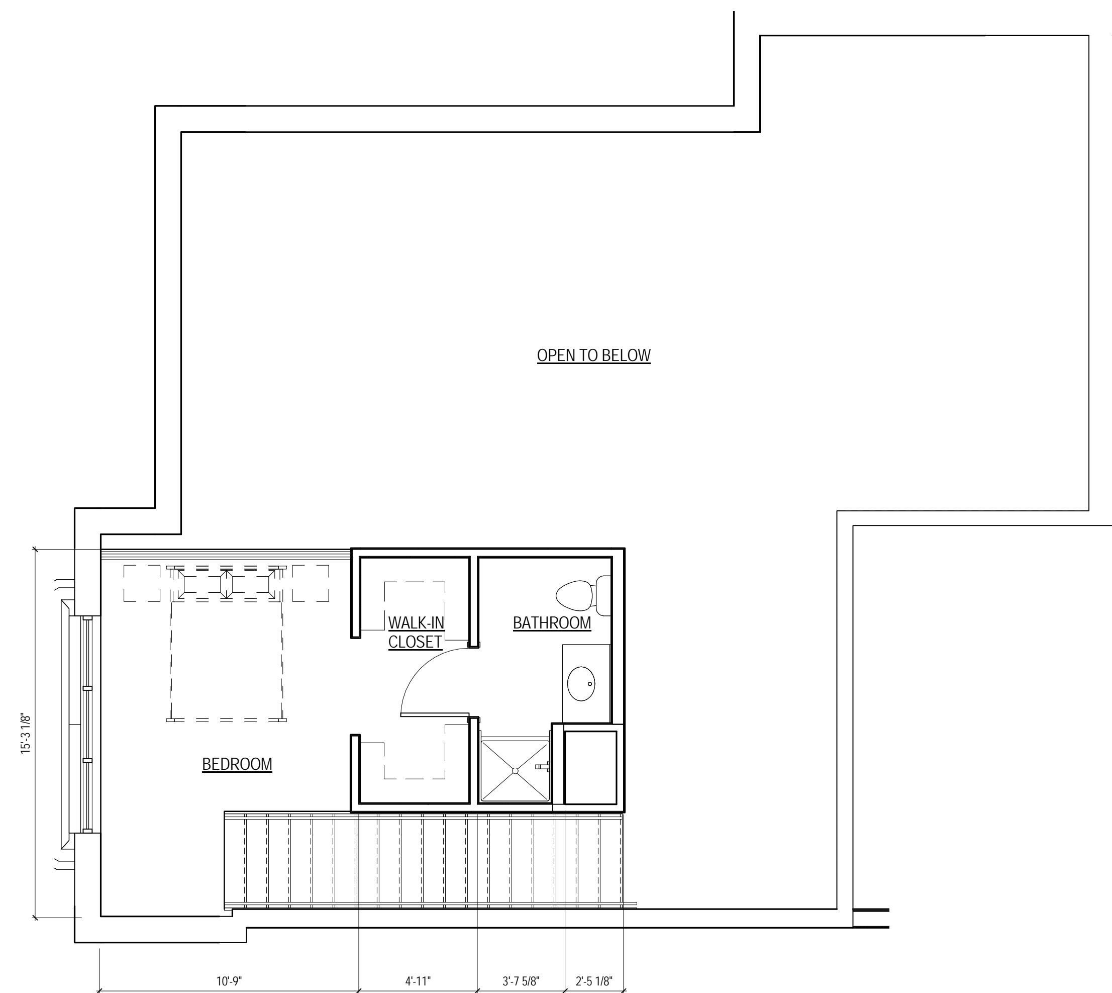
6 LOFT UNIT C - SECOND FLOOR A 233 1/4" = 1'-0"
