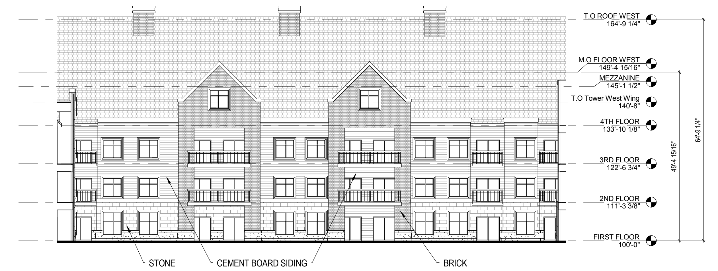
5 West Elevation - Court Yard A 401 1/16" = 1'-0"
