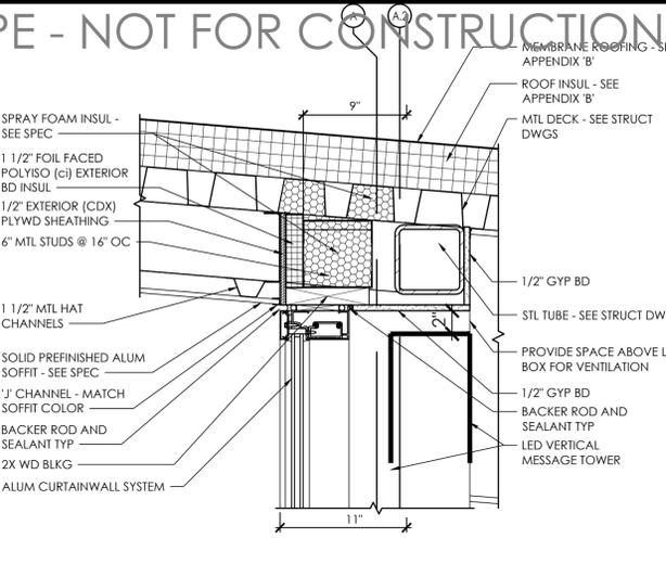
**B3** Exterior Section Detail - Vertical Message Tower Head
