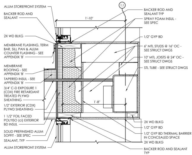
**C2** Exterior Section Detail - Canopy Roof at Storefront
