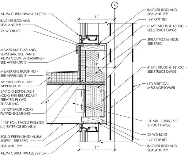
**B2** Exterior Section Detail - Vertical Message Tower Head & Sill
