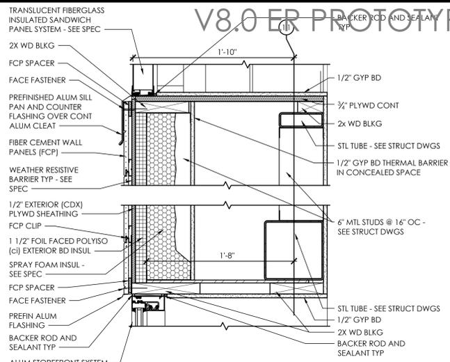
**C3** Exterior Section Detail - Translucent Panel Sill/Storefront Head
