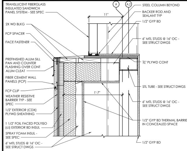
**D3** Exterior Section Detail - Translucent Panel Sill
