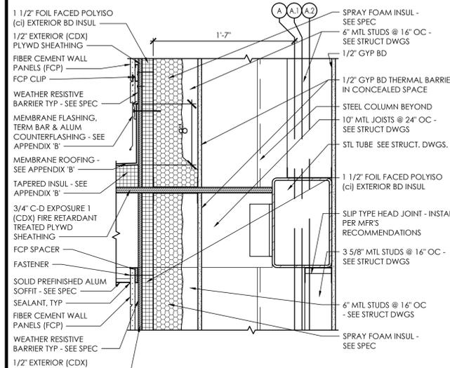
**D2** Exterior Section Detail - Canopy Roof at Fiber Cement Panel
