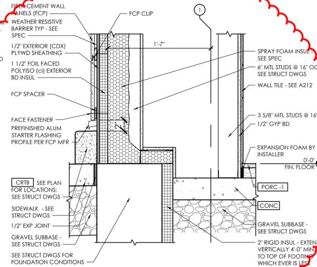
**A1** Exterior Section Detail - Fiber Cement Wall Pnl Base of Curb
