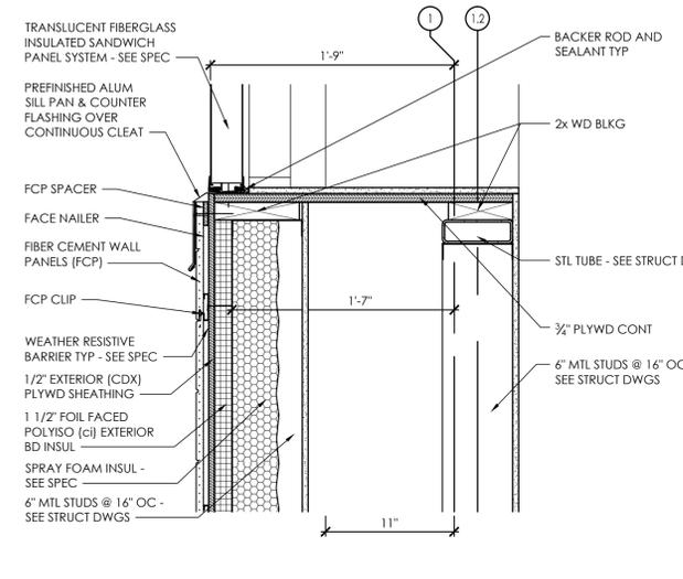
**A2** Exterior Section Detail - Translucent Panel Sill
