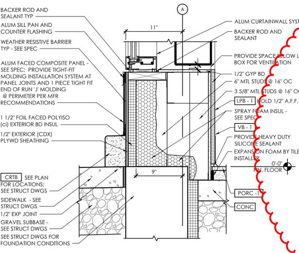
**B1** Exterior Section Detail - Vertical Message Tower Sill
