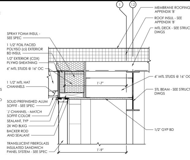
**A3** Exterior Section Detail - Translucent Panel Head
