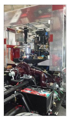
Access to the pump will be provided by raising the cab. The pump will be positioned such that all maintenance and overhaul work can be performed above the frame and under the tilted cab. The service and overhaul work on the pump will not require the removal of operator panels or pump panels. Complete pump casing and gear case removal will require no more than removal of the intake and discharge manifolds, driveline, coolers and a single discharge line. The pump case and gear case will
