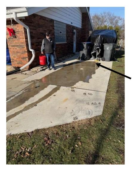
Water drainage testing. ½ full bucket of water.
