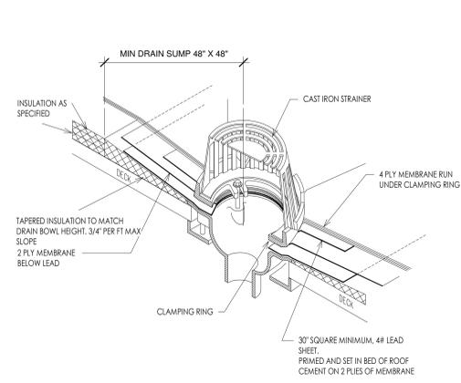
4 ROOF DRAIN DETAIL
