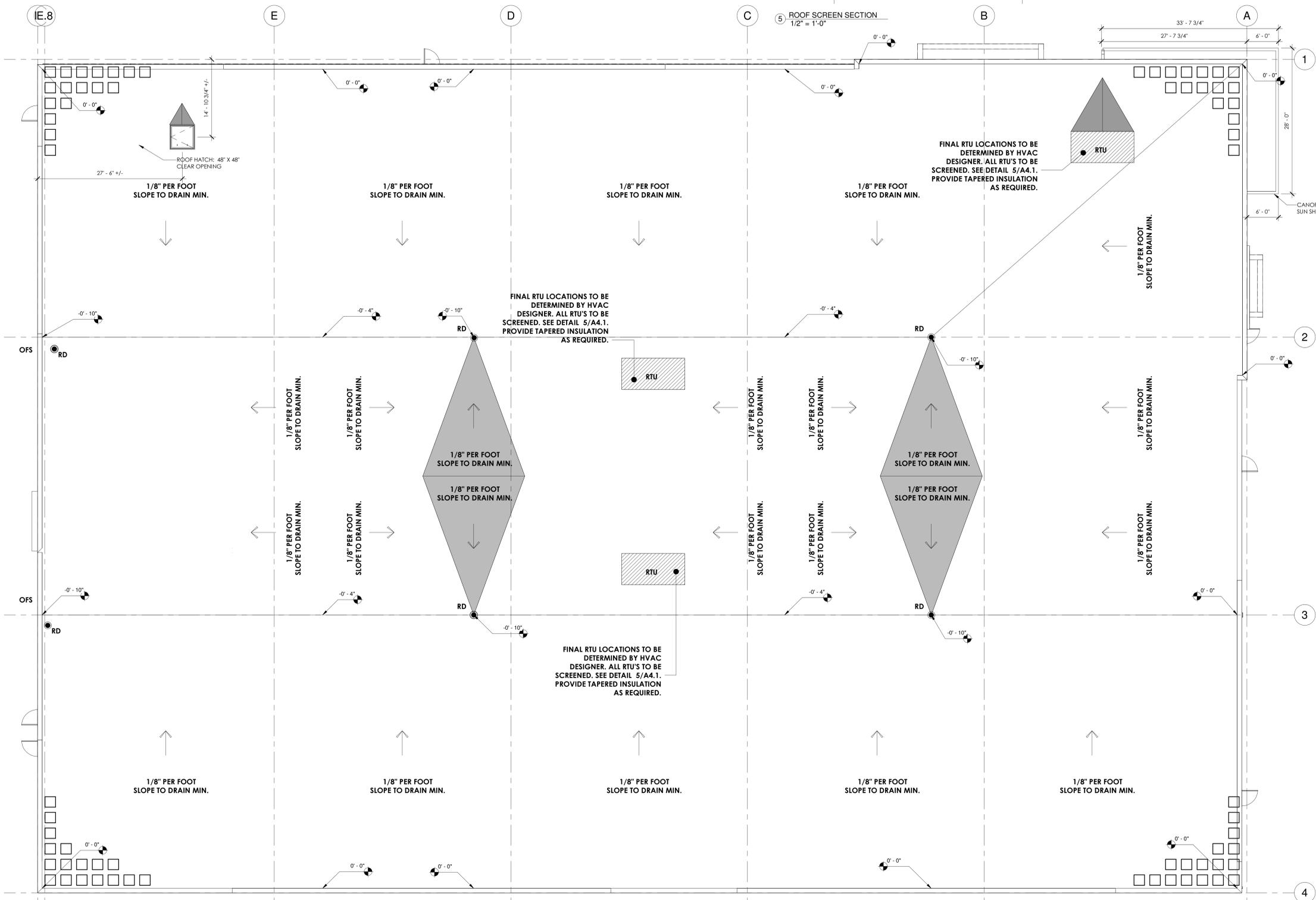
PROVIDE ROOF PAVERS AT ROOF HATCH AND AT ALL ROOF TOP UNITS. REFER TO HVAC PLANS FOR EXACT LOCATION.
