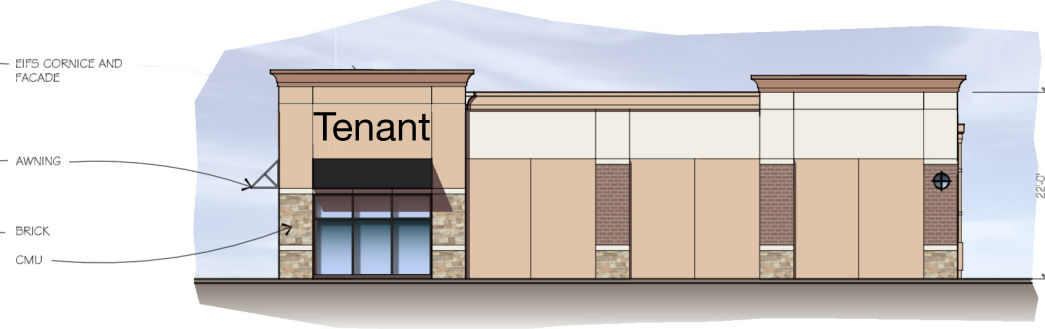
BUILDING E NORTH ELEVATION SCALE: 3/32"=1'-0" 5 A4.4
