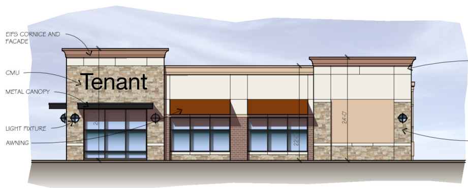
BUILDING F NORTH ELEVATION SCALE: 3/32"=1'-0" 4 A4.4
