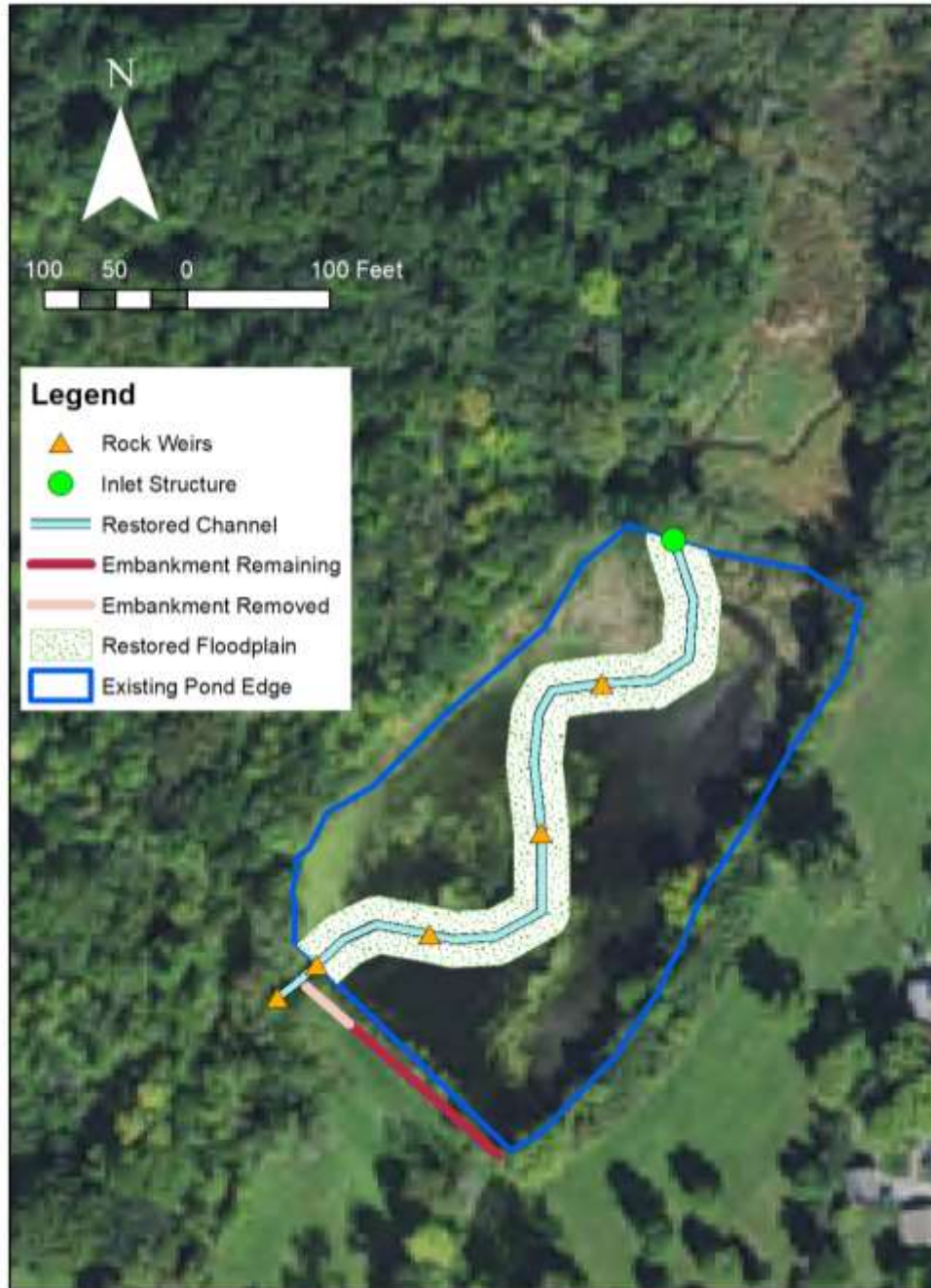
Figure 7. Alternative 2 - Remove Dam and Restore Creek
