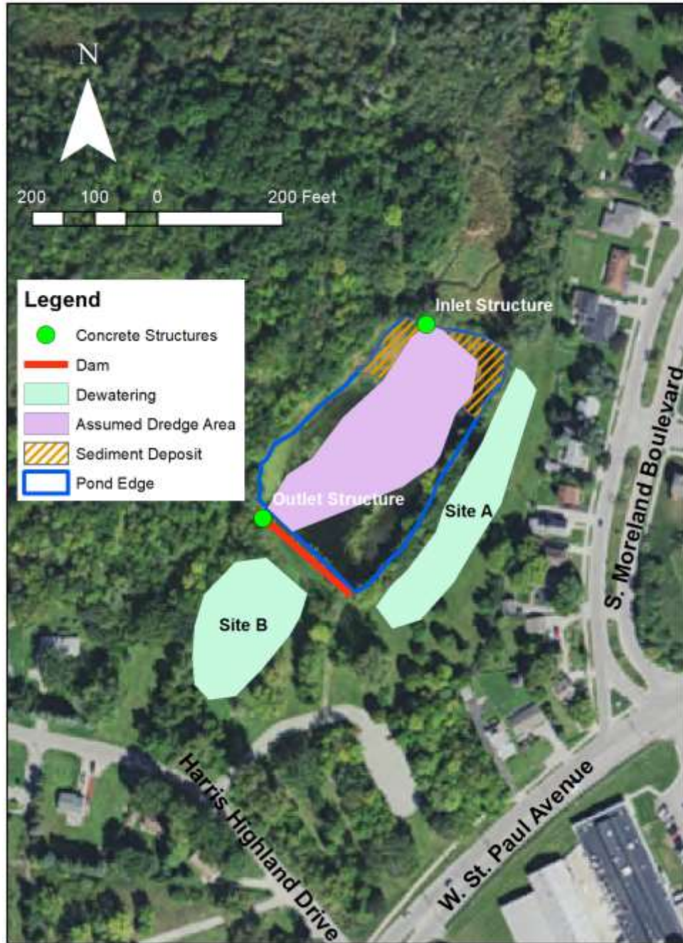
Figure 6. Alternative 1 - Repair Dam and Dredge Pond
