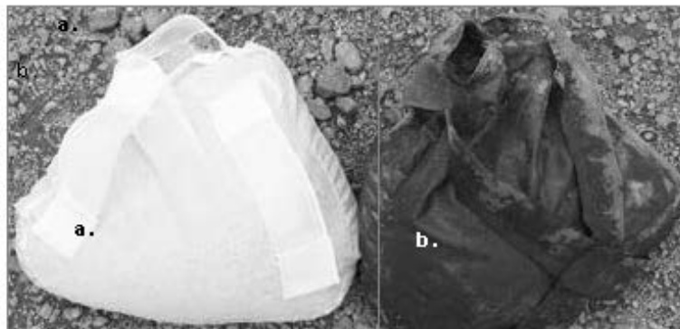
Fig. 4 a) A new Media Bag of Hydro Filter Sand. b) A spent media bag of Hydro Filter Sand.
