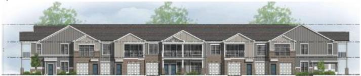
This elevation includes more wainscotting along the base of the elevation as well as increased masonry within recessed articulations to provide more of the look that was discussed during the concept hearing.
