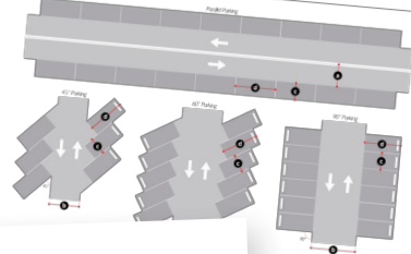
Graphic 10.2: Dimensional Standards for Parking Spaces and Aisles
