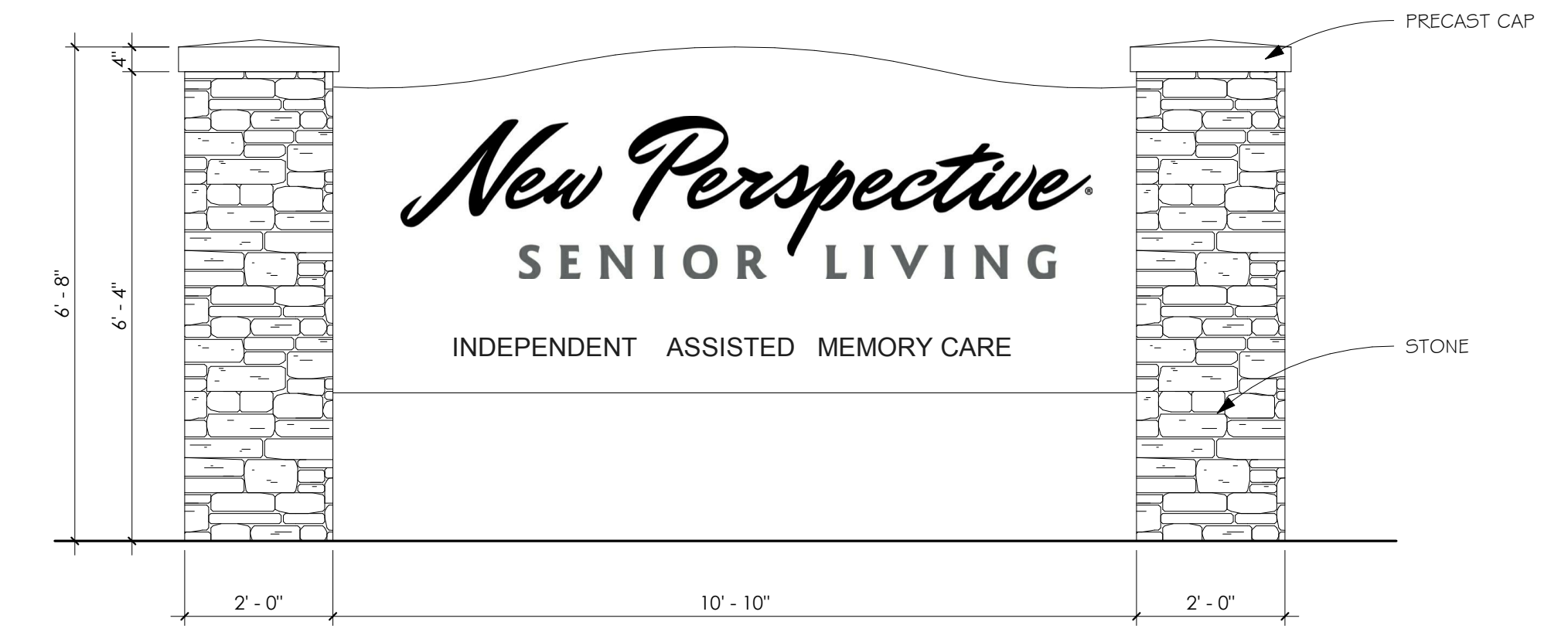
2 MONUMENT SIGN ELEVATION SCALE 1/2" = 1'-0"
