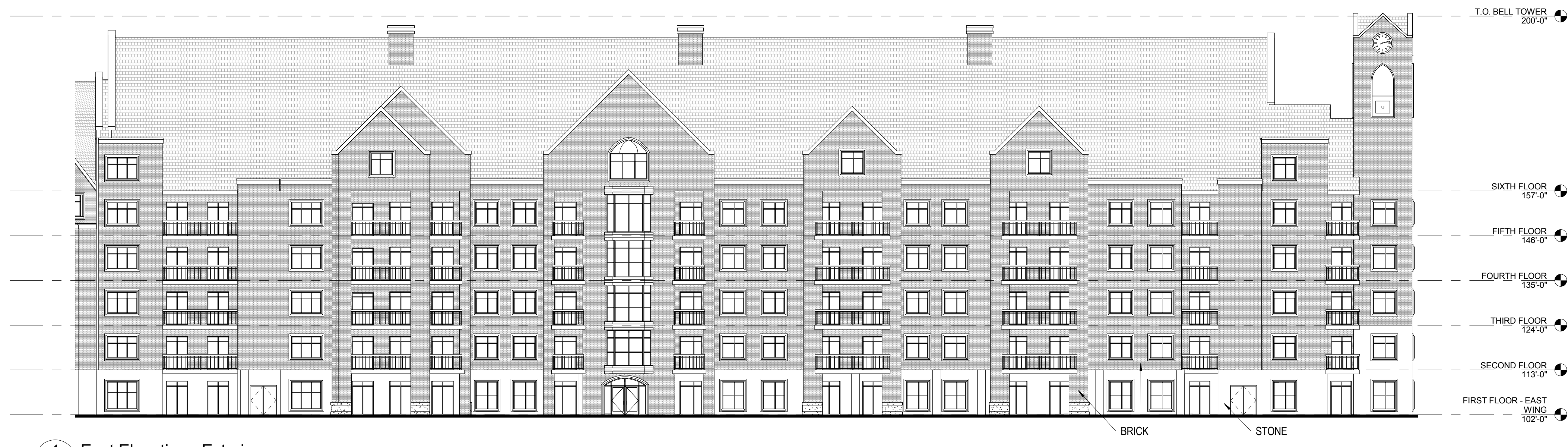
1 East Elevation - Exterior A 402 1/16" = 1'-0"
