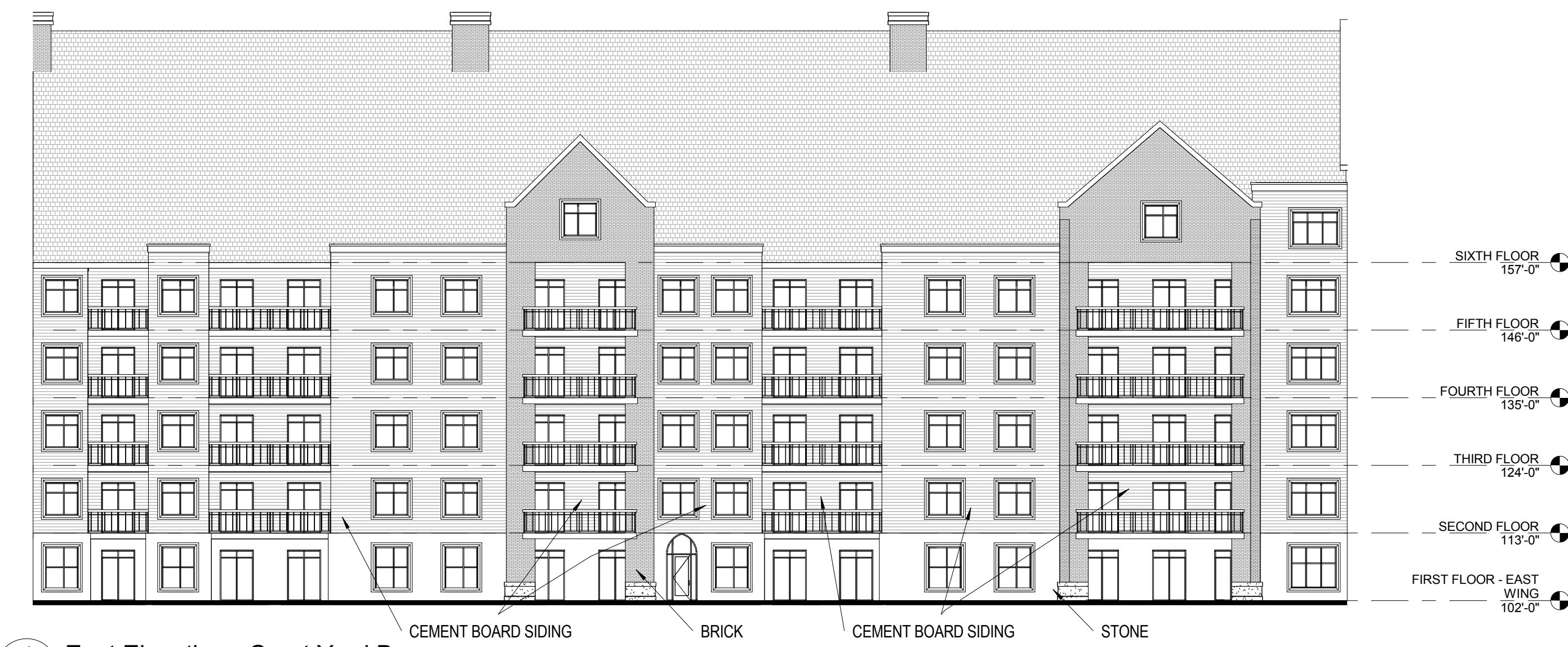
4 East Elevation - Court Yard B A 402 1/16" = 1'-0"
