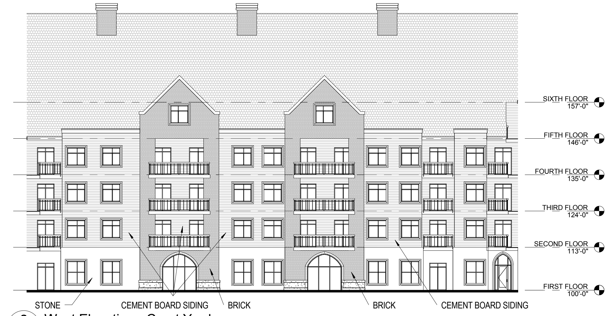
2 West Elevation - Court Yard A 401 1/16" = 1'-0"
