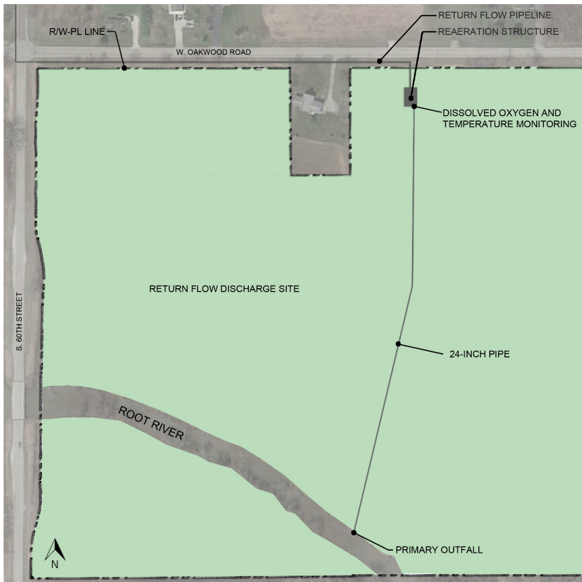
Figure 11. Return Flow Discharge Site Facilities Locations
