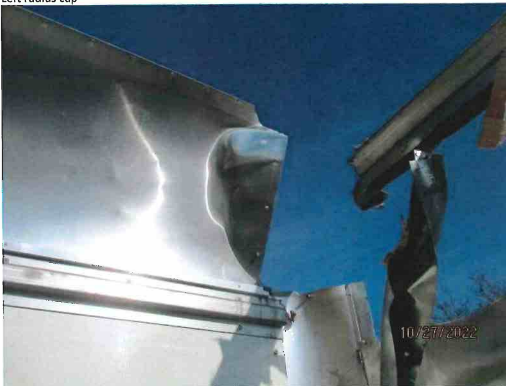
Right radius cap missing
