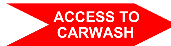
NON-LIT DIRECTIONAL SIGN WHITE VINYL ON RED ALUMINUM 1'-0"H X 4'-0"W = 4.0 SQ FT
