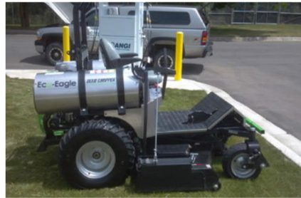
Lawn mower retrofit to operate on CNG.
