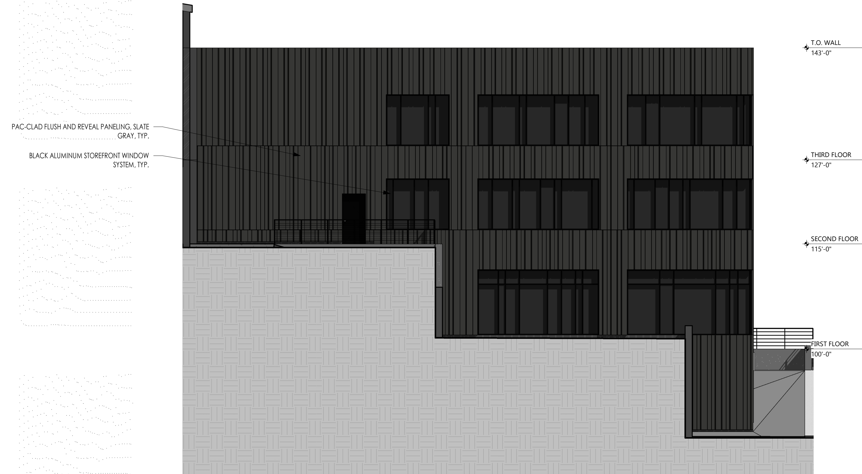
② ADDITION SOUTH ELEVATION 1/8" = 1'-0"
