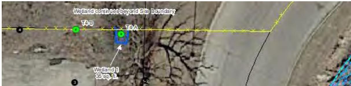
Wetland 1 would be considered **E2Kx** (emergent/wet meadow, narrow-leaved persistent with wet soil, palustrine, excavated). The wetland boundary for Wetland 1 is located along a topography break within an excavated ditch. The wet meadow receives stormwater from a culvert which empties into the ditch. The wetland meets wetland criteria for hydrophytic vegetation, hydric soil, and wetland hydrology.
