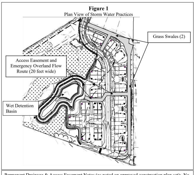
Permanent Drainage & Access Easement Notes (as noted on approved construction plan set): No building, filling or grading changes allowed in the Permanent Drainage & Access Easement.
