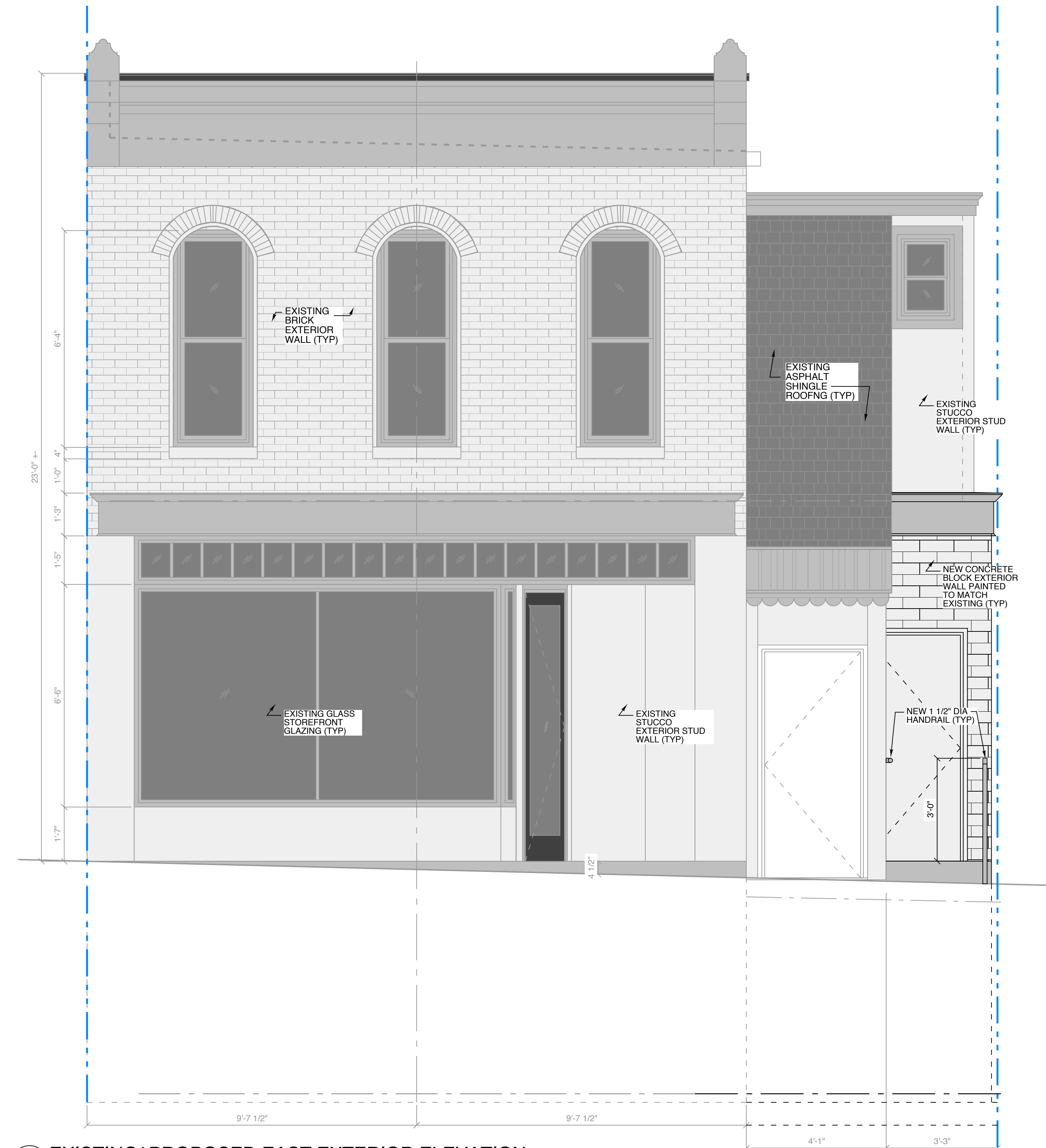
3 A2 EXISTING/ PROPOSED EAST EXTERIOR ELEVATION SCALE: 1/2" = 1'-0"
