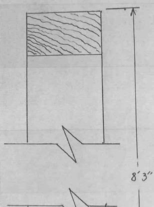
Standard 2x4 nonbearing wall construction ranging in hights up to 8:33 16 on center determined by height and location to roof Some walls will have drywall on 2 sides some on I side
