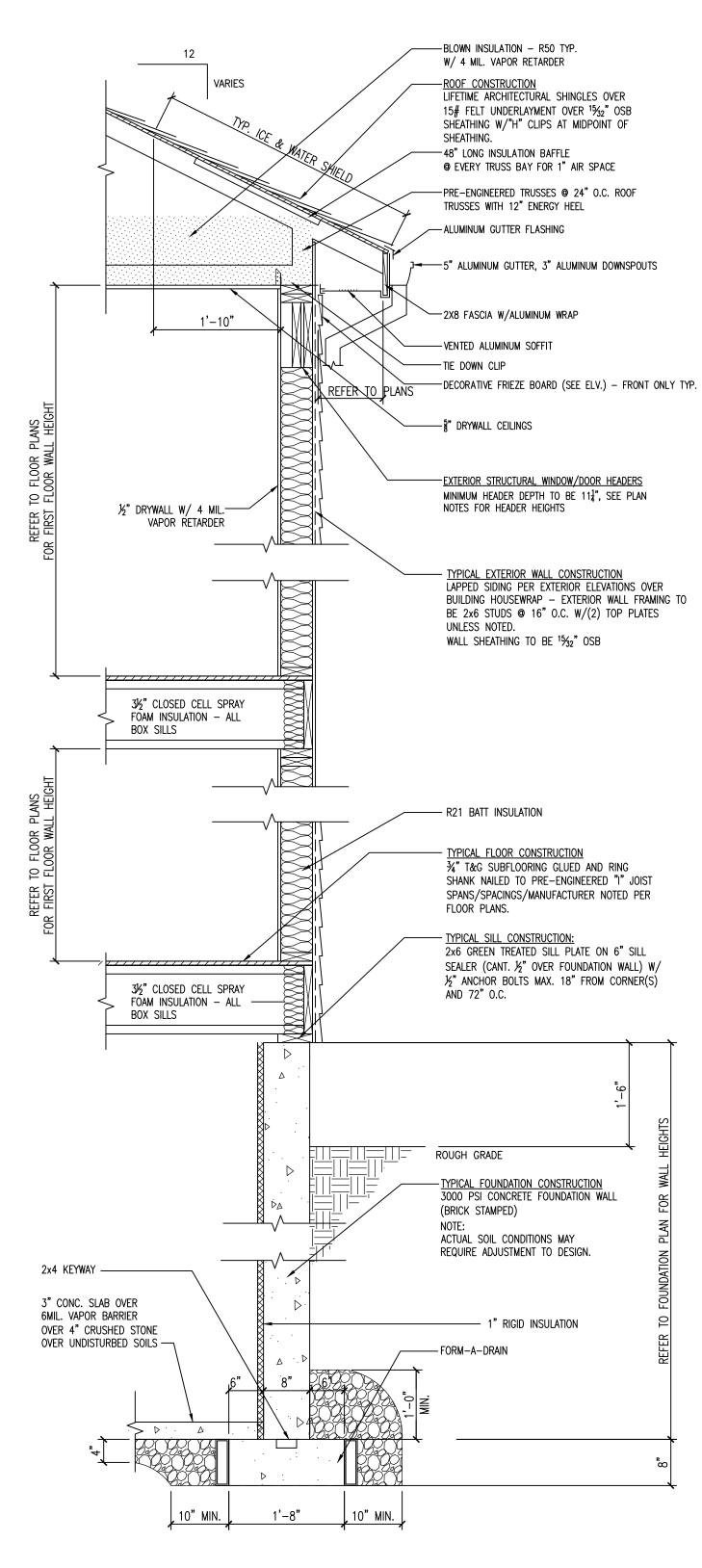
SINGLE STORY WOOD FRAME WALL - 9'-4" FOUNDATION WALLS TYPICAL WALL SECTION 3/4" = 1'-0" SCALE:
