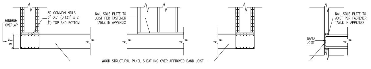
OVER RAISED WOOD FLOOR OR SECOND FLOOR - WOOD STRUCTURAL PANEL OVERLAP OPTION
