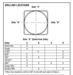
Note: Standard SF and DF pole preparations are located 3/4 of the height of the pole from the base, unless otherwise specified.
