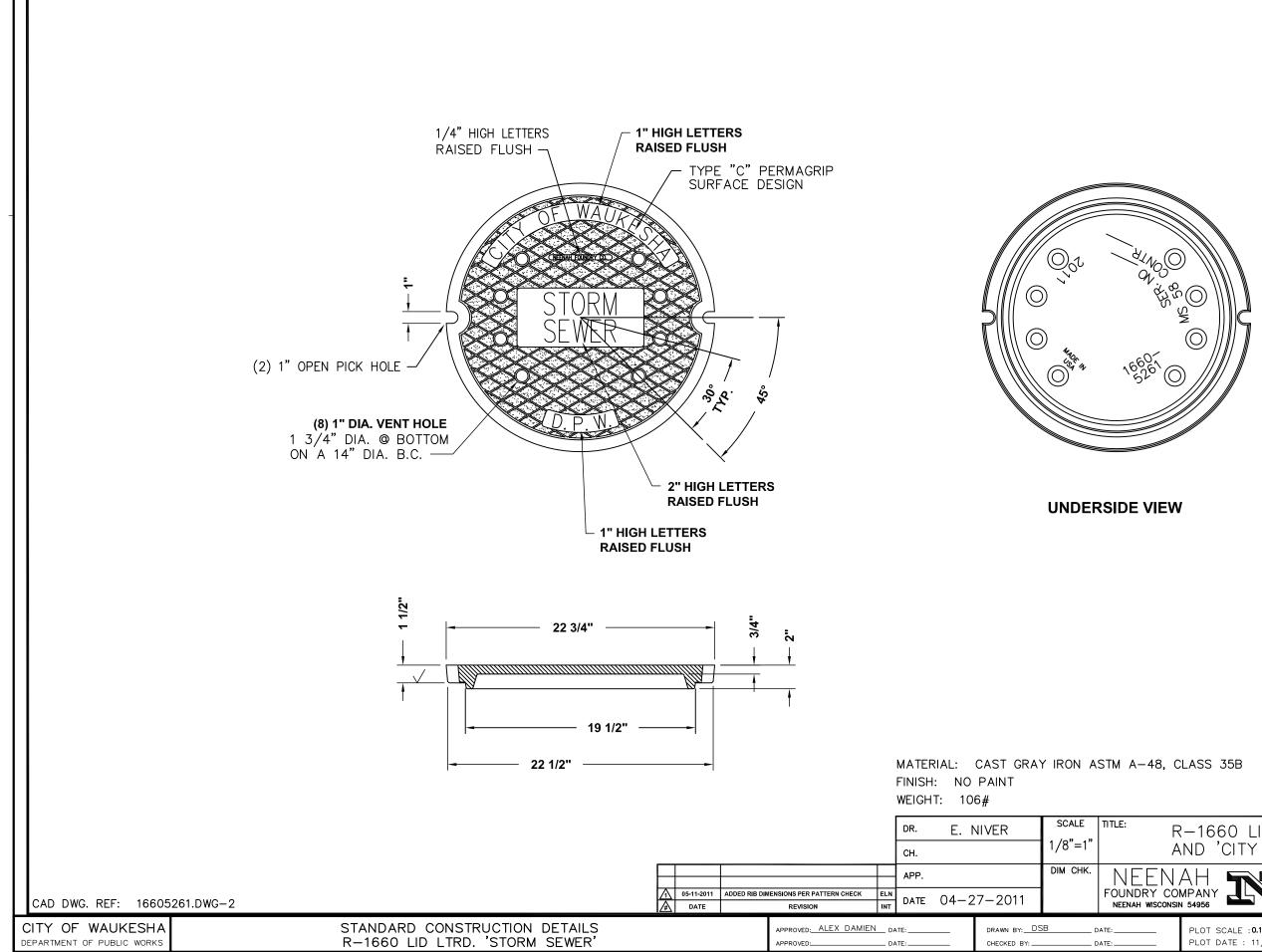
R-1660 LID LTRD. 'STORM SEWER' AND 'CITY OF WAUKESHA', 'D.P.W.' **NF-**16605261 В DETAIL NUMBER: 05-1660 PLOT SCALE :**0.123430** PLOT DATE : 11/21/2017 2:59 P STANDARD DETAILS PROJECT NO:
