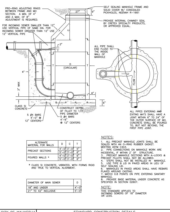
STANDARD CONSTRUCTION DETAILS CITY OF WAUKESHA STANDARD DROP MANHOLE DEPARTMENT OF PUBLIC WORKS Ш DETAIL NUMBER: APPROVED: ALEX DAMIEN DATE: DRAWN BY: JAW 05-0005 DATE: PLOT SCALE :0.700000 CHECKED BY: DATE: PLOT DATE : 11/27/2017 7:33 AM PPROVED: DATE: PROJECT NO:
