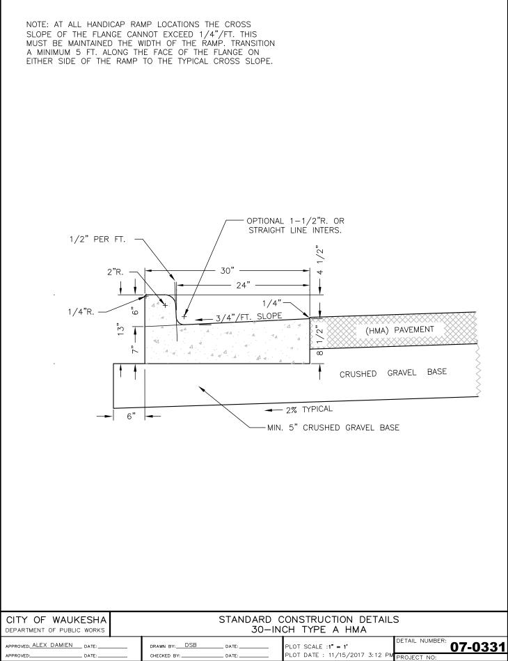
FILE NAME : 0: \\_PROJECTS\Standard Specifications\Standard Details\Final\07-0331-30 INCH TYPE A HMA.dwg
