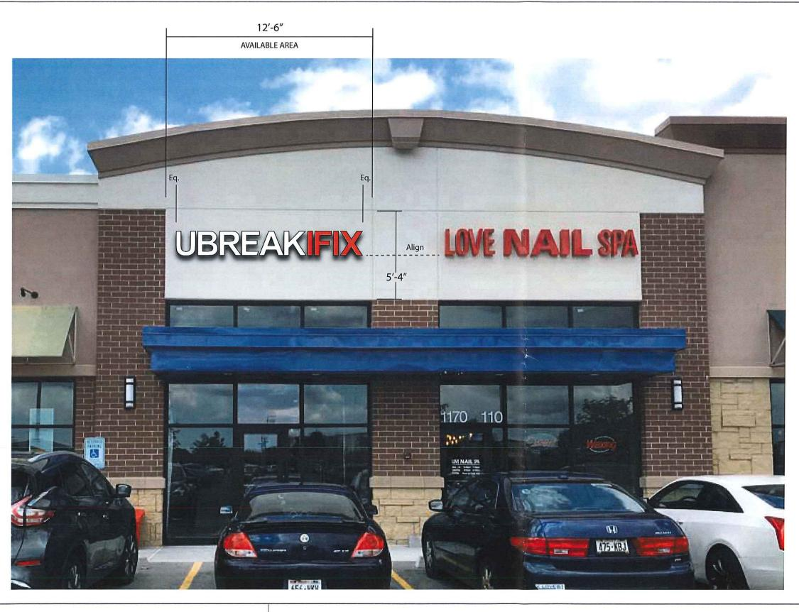
09-04-18 (ZW) Job # 1846-0752 PRODUCTION DRAWING Channel Letters - Individually Mounted One (1) Set of Face Lit Channel Letters Individually Mounted Illuminated with internal white LED Sign to have Photo Cell (A) Returns: 5" deep .040 letter coil - Black (B) Trim Cap: 1" black (C) Face: .177 white acrylic (D) Graphics: 3M film applied to 1st surface Installation Method: Mounted flush to exterior wall. (verify) Colors: White (acrylic) Red (acrylic #2415)
