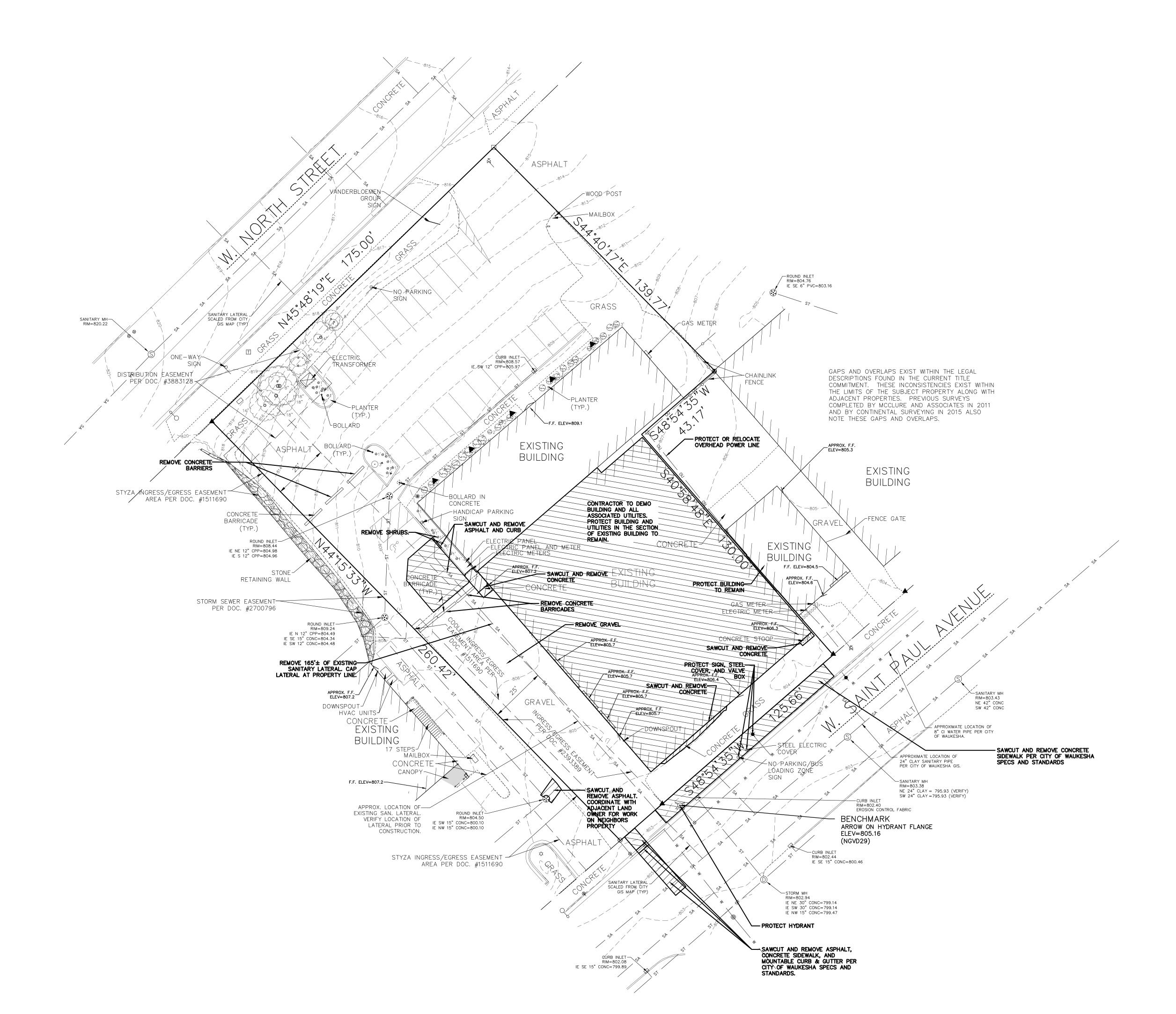
CONTRACTOR TO TELEVISE ALL SANITARY LINES TO DETERMINE SANITARY ROUTING AND LOCATION OF CONNECTION(S) INTO THE PUBLIC MAIN. REMOVE ALL SANITARY LÀTÉRALS TO THE PROPERTY LINE AND CAP. CONNECT EXISTING STORM SEWER TO REMAIN INTO THE PROPOSED LATERAL OR THE INTERIOR SANITARY.
