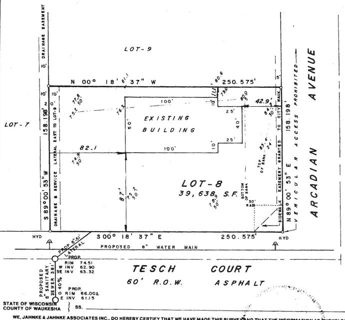
WE, JAHNKE & JAHNKE ASSOCIATES INC., DO HEREBY CERTIFY THAT WE HAVE MADE THIS SURVEYAND THAT THE INFO THE ABOVE PLAT OF SURVEY IS TRUE AND CORRECT REPRESENTATION THEREOF. Revised 4/2/98 (Stakeout)
