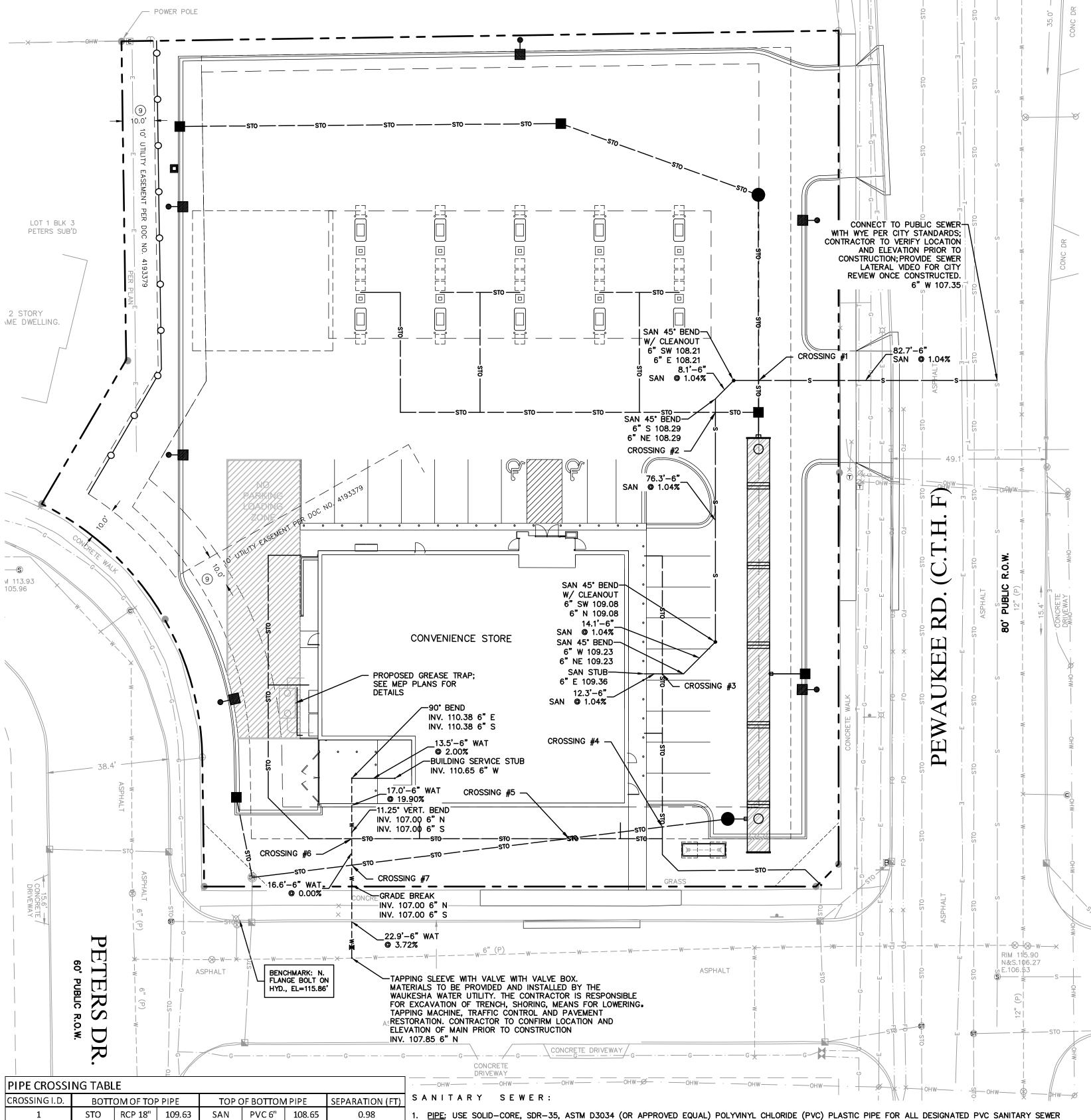
INSTALLATION MUST COMPLY WITH ASTM D2321.
