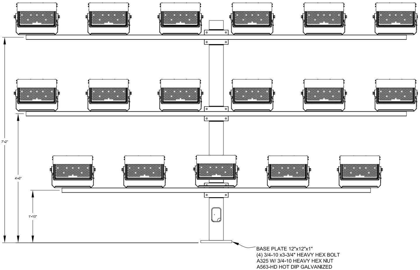
\*\* Hot-Dip galvanized after fabrication to ASTM A123 specifications
