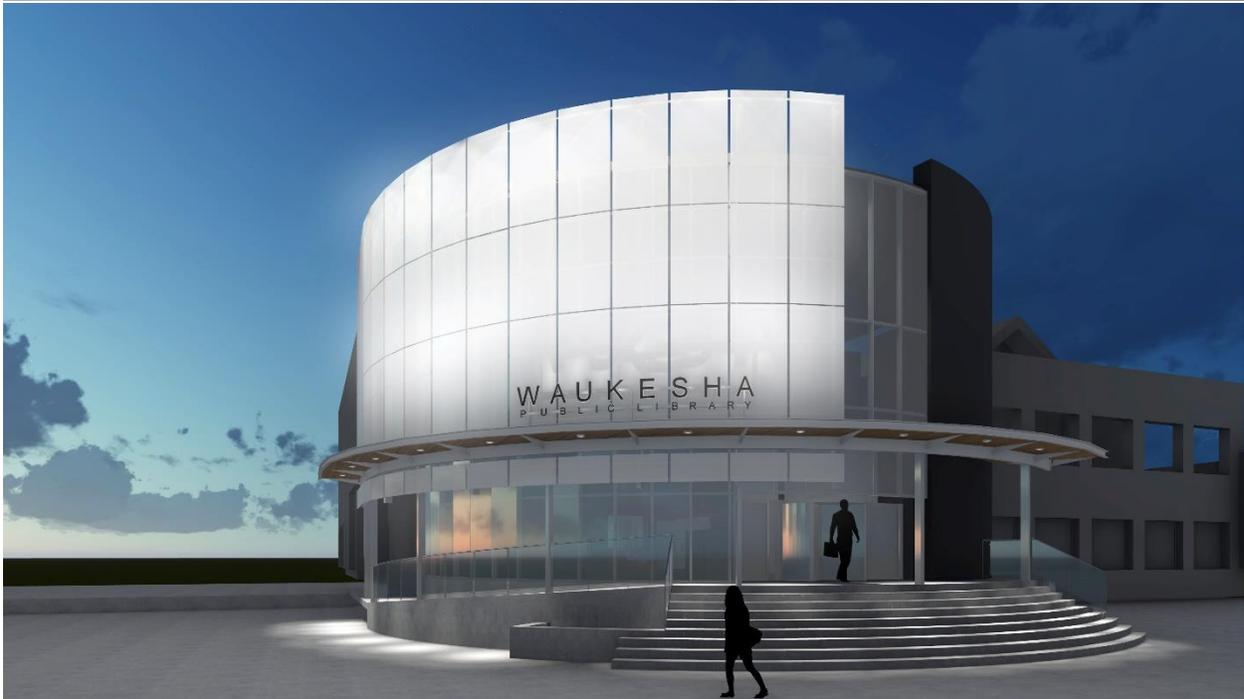
3. These are two night views of the images from the previous page—(above) with horizontal resin panels and (below) with a horizontal canopy. Note the effect of the lights attached to the horizontal panels in the second image.
