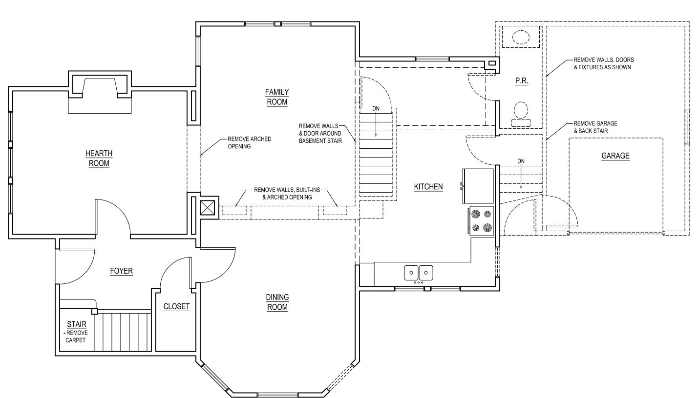
EXISTING / FIRST FLOOR DEMOLITION PLAN
