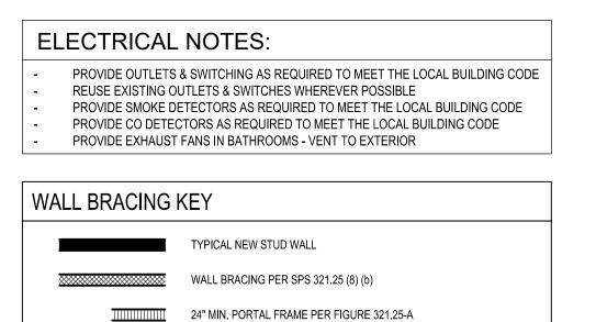
NOTE: PROVIDE 4'-0" LINEAR BRACING WHERE POSSIBLE UNLESS NOTED OTHERWISE
