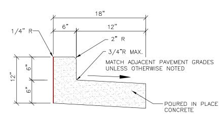
18" REJECT CURB & GUTTER DETAIL
