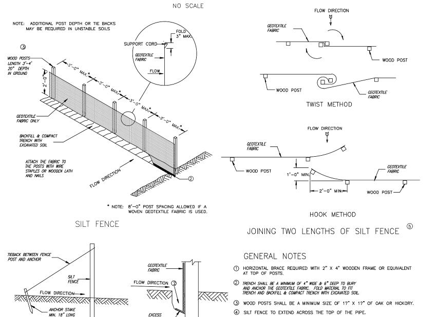
SILT FENCE INSTALLATION DETAIL NO SCALE
