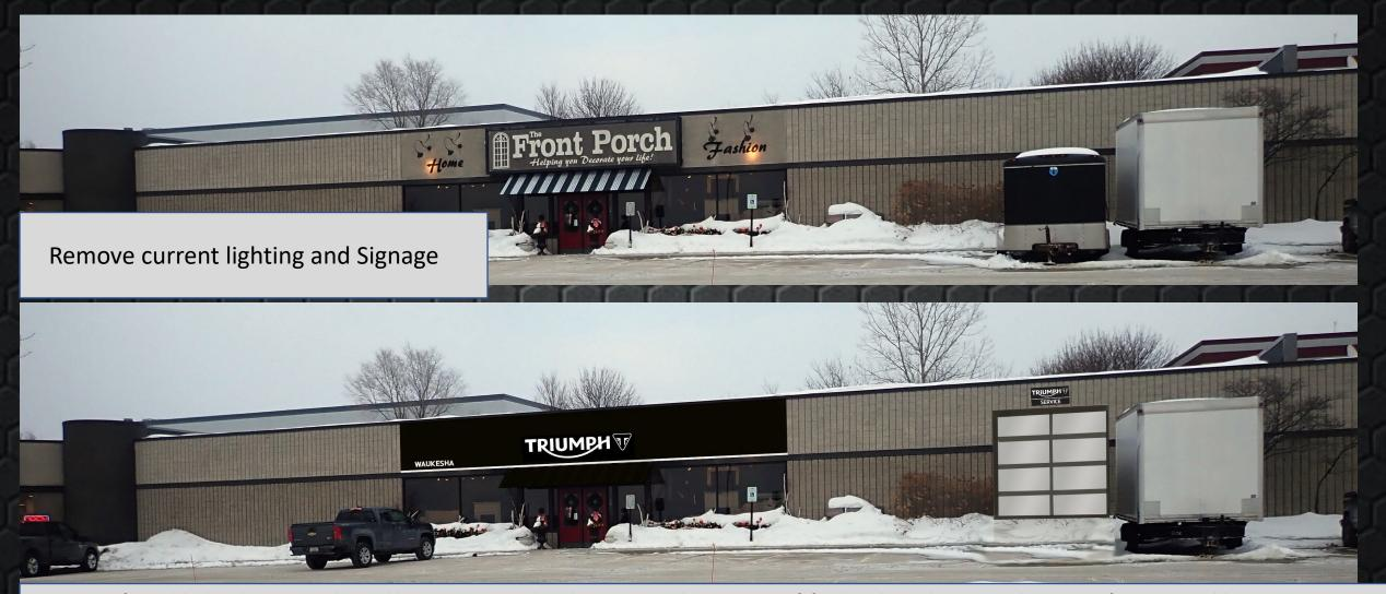
Painting fascia black, adding new channel letter signage, white line is painted. See SignArt® for details on dimensional aspects of signage. Adding service sign on far right. All lights are back lighted. Dealer to add roll-up door for service – New aluminum framed glass overhead door.
