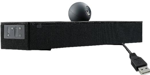
To use the camera and microphone, connect your laptop to the AMX Conferencing System using the USB cable.
