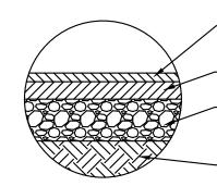
1.75" SURFACE 4LT52-28S OVER TACK COAT 1.75" BINDER 4LT52-28S (LOWER LAYER) 8" DENSE GRADE AGGREGATE BASE COURSE (1-1/4")
