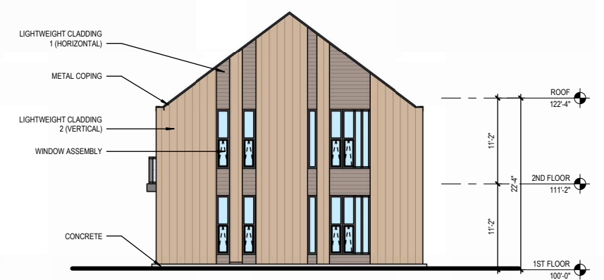
WEST ELEVATION - BUILDING D/E
