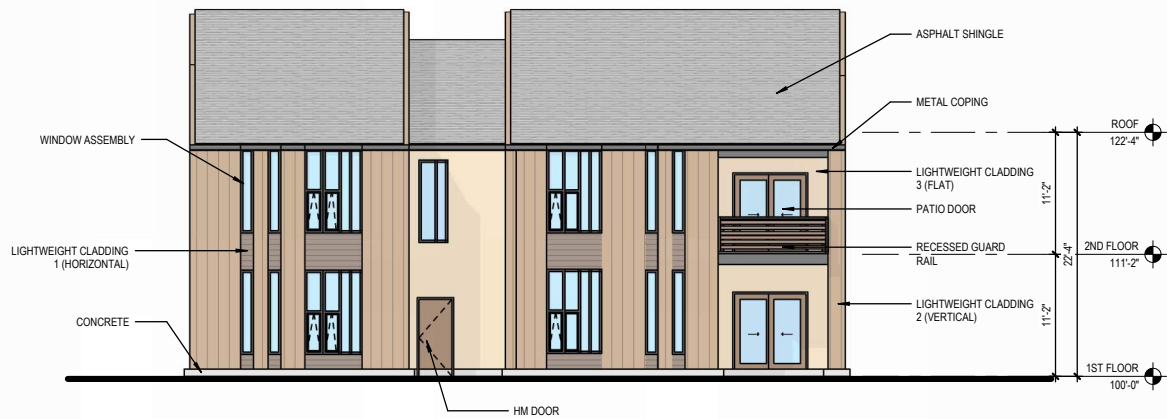
SOUTH ELEVATION - BUILDING D/E
