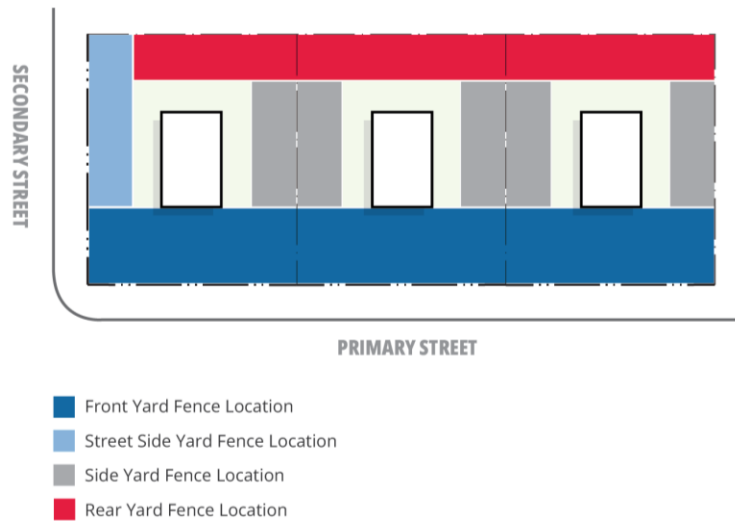
Figure 1 Lot Fence and Wall Configuration - Location
