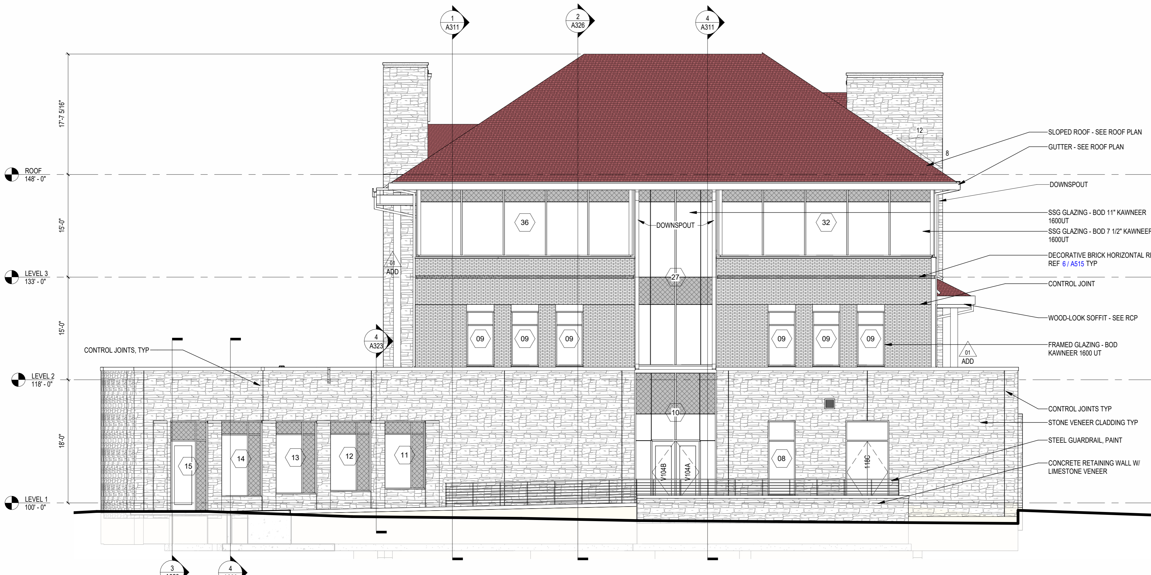
2 EXTERIOR ELEVATION - NORTH 1/8" = 1'-0"
